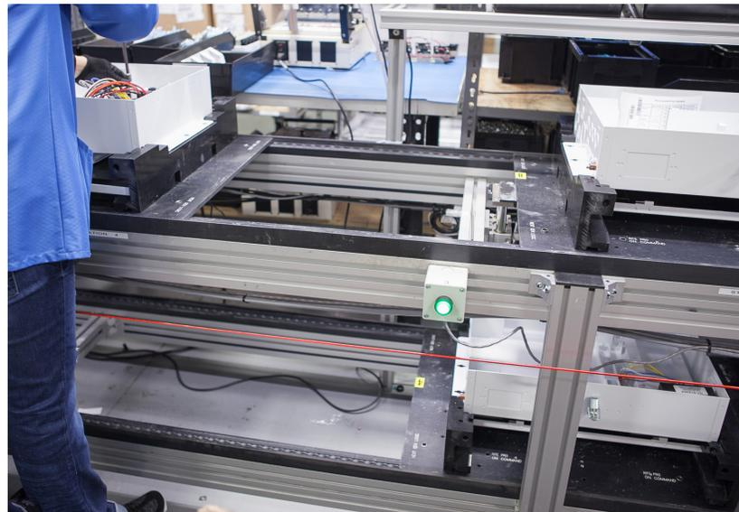
Over-under systems are useful when floor space is at a premium. Vertical transfer units are used to move the pallet, with or without product; between the different conveying levels.
